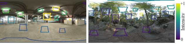
Figure 6: Visualization of optimized light parameters on an environment map. The light's area is visualized as the rectangle size, while the rectangle color indicates the light's intensity.
