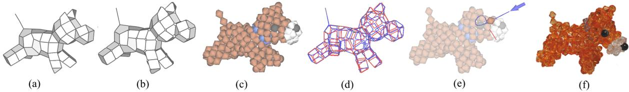
**Figure 1:** System overview. (a) The user creates a design model. (b) The system runs a simulation on a structure model to adjust the geometry. (c) The beadwork model visualizes the expected result. (d) The system computes the wire path. (e) The system provides a step-by-step construction guide. (f) The user manually constructs a physical beadwork.
