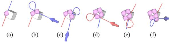
**Figure 3:** An example of the visual construction guide. (a) Initial state. (b,c,f) Blue wire passes a newly added bead. (d) Red wire passes a newly added bead. (e) Red wire passes an existing bead.
