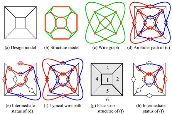
**Figure 4:** Details of the wire path-planning algorithm. Yellow beads are stable beads and pink beads are unstable beads.
